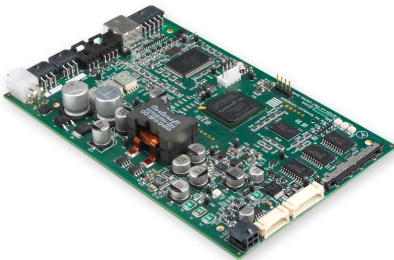
Meteor HDC-K datapath and driver board for Kyocera KJ4 printhead
